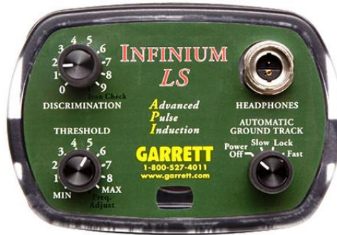
Infinium LS control panel
