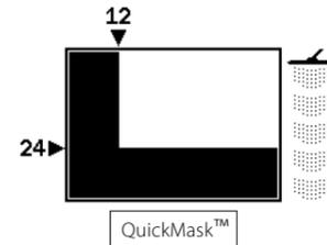
QuickMask™ has two slider controls to adjust the level of Ferrous and Conductivity discrimination.
