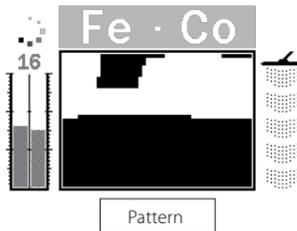
Target information is presented to you via the Smartfind™ Discrimination Pattern, Sensitivity Gauge, FE-CO numbers and Depth Gauge.
